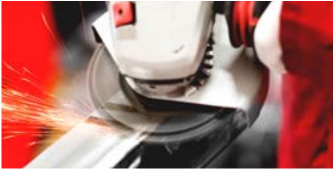
Grinding with Zebra slotted see-through disc: good view of the material being processed.
