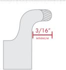
**Rim Flange Depth** Some wheels feature rim flanges that are not intended for clip-on wheel weights and are only added for decoration purposes. All rim flanges that are less than 3/16" deep should utilize an adhesive wheel balance weight.
