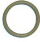
Art. No. 469.09015 ID: 0.551" | 14mm OD: 0.691" | 17.56mm Thickness: 0.067" | 1.7mm
