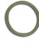
Art. No. 469.902110 ID: 0.551" | 14mm OD: 0.724" | 18.38mm Thickness: 0.09" | 2.29mm
