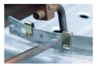
The powerful force of the fixing clamp keeps the clamped sheet metal in place.
