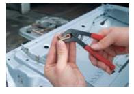
1. Insert the fixing clamp into the special pliers and open the clamp.
