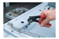
2. Slide the clamp over the sheet metal edges to be joined and release the pliers.
