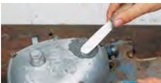
Repair of small-size engine cover
