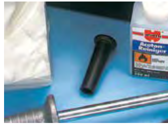
Adapter Installation Tool Art. No. 691.500114 - Qty. 1 For safe installation and removal of the adapters
