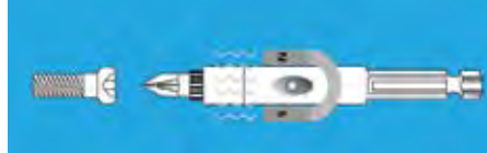
The strong magnet will magnetize the bit, securing a firm hold of the screw.
