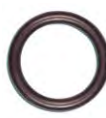
Art. No. 469.211 ID: 13/16" | 20.638mm OD: 1-1/16" | 26.988mm Thickness: 1/8" | 3.175mm
