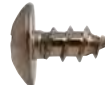
VW, Audi Art. No. 140.70603 - P. Qty. 100 #10 x 3/8 Truss Head PH SMS License Plate Screw, 18.8
