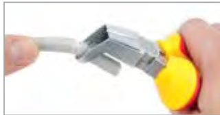
Bend the cable end slightly until the separation point breaks, and pull off the piece of sheath
