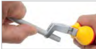
Carefully cut into the sheath with the blades until the stop rests against the sheath. Then rotate the pliers part way around the cable
