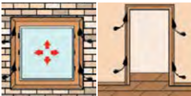
Installation of windows and doors
