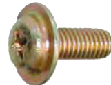
Ford Contour & Mercury Mystique 1995 - on Art. No. 140.7050 - P. Qty. 100 Zinc & Yellow Dichromate, PH pan washer head, M5 - 0.8 x 12mm 12.7mm washer head O.D.
