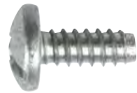
GM Art. No. 140.19777 - P. Qty. 50 Dacromet 320, M6.3-1.81 x 16mm (#14 x 5/8"). Duo drive truss head license screw, 14mm head O.D.
