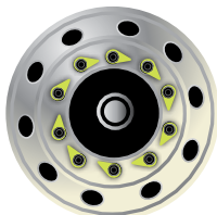
Front view of wheel with wheel flags on all nuts
