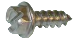
Universal Art. No. 140.7070 - P. Qty. 100 1/4 x 3/4" Hex Washer Head Slot Type 'A', 18-8 Stainless Steel, use with License Plate Nut Art. No. 140.6000
