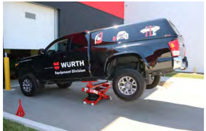
Both images above showing SUV Frame adaptors, Art. No. 995.103FA , in use.
