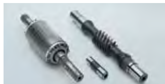
Bearing seats, repaired and then reworked
