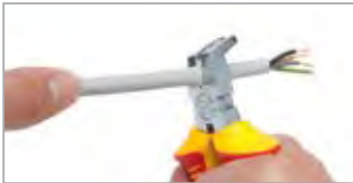
Cut cable with the side cutter
